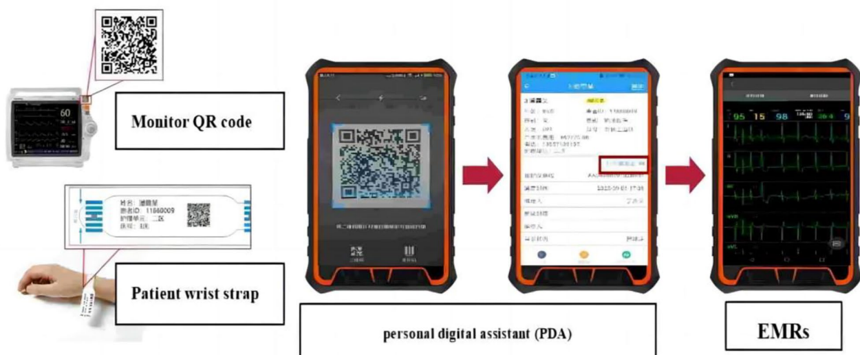
Fig. 1 ICU nursing electronic medical record is linked with the monitor, real-time receiving patients’ vital signs data
