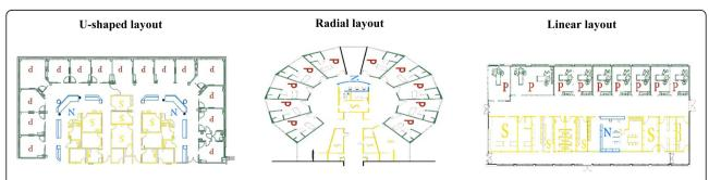
**Fig. 1** Common examples of centralized nurse station and ward layout. (P represents patients' rooms, N the nurse station, and S service and support spaces)
